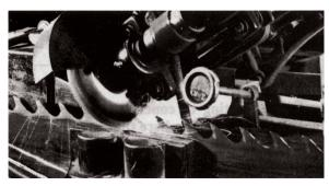
Illustration 13 – Sharpening teeth (saw gumming) on a large band saw
